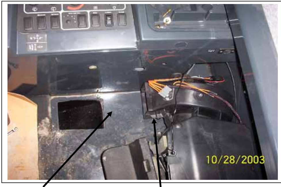
Air outlet channel removed
